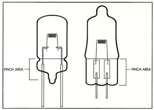
This illustration of the two types of typical halogen cycle lamps, the one on the left employing General Electric aluminosilicate glass and the one on the right using fused quartz or 96% silica glass, can be used to compare the merits of the two materials. With these GE aluminosilicate glasses, lead wires can be single lengths or two part round leads with one weld per lead, rather than assemblies of wire
