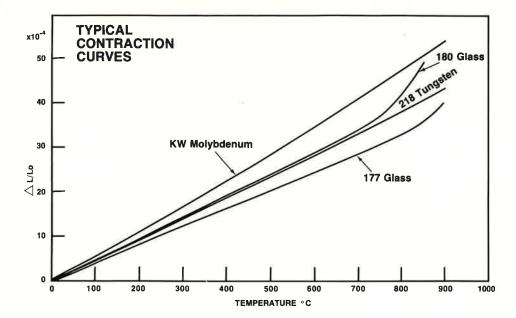
Glass expansion coefficients are normally given for the temperature range 0-300°C. However, understanding of stresses in glass-to-metal seals requires knowledge of the contraction coefficients of the materials from the setpoint of the glass to room temperatures.
